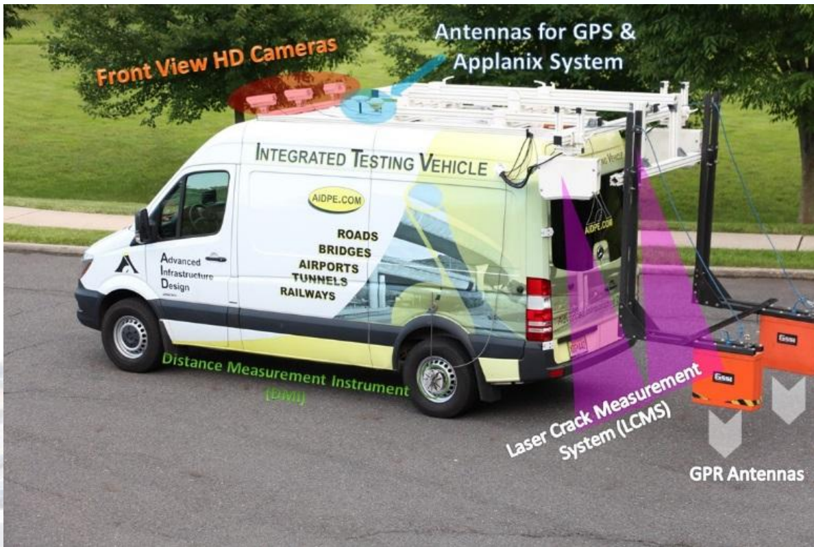
AID's ITV Equipped with LCMS, HD Cameras, GPR, and GPS w/Applanix
