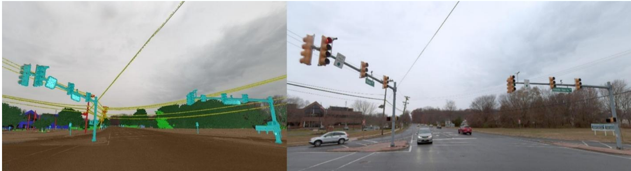
Sample mobile LiDAR point cloud dataset (left) and sample synchronized panoramic imagery (right)
