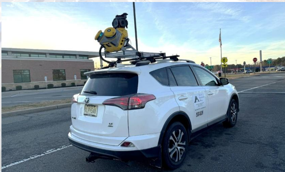
AID testing vehicle equipped with mobile LiDAR system
